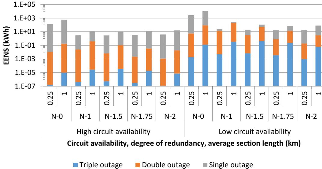
Figure 11.3: EENS for different circuit availabilities, degrees of redundancy and section lengths for underground feeders with total feeder peak demand of 2,500 kW; logarithmic Y-axis
