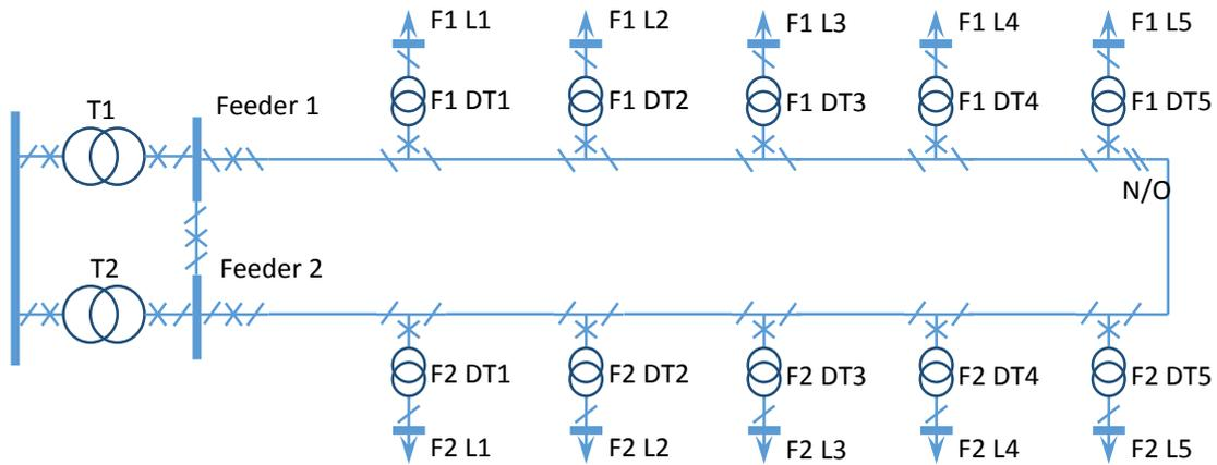
Figure 9.19: An example of radial HV distribution network
