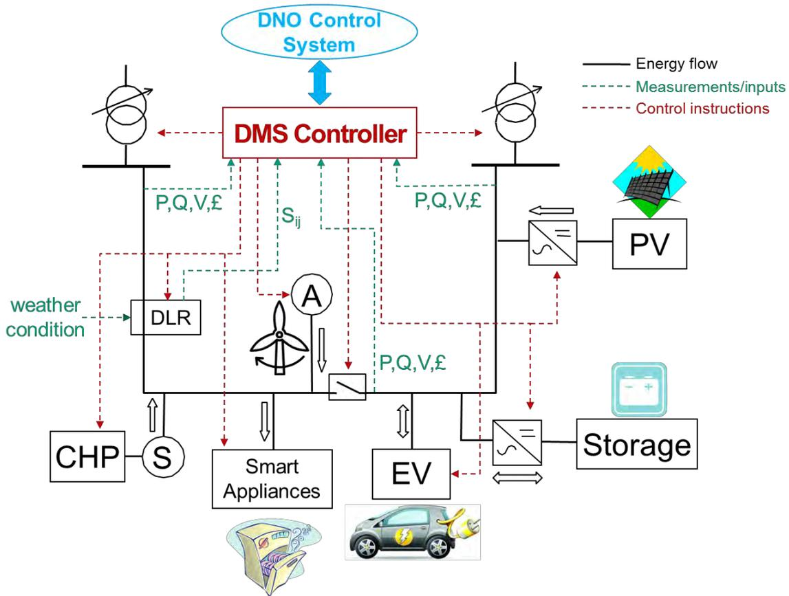
Figure 6.1. Active distribution network operation
