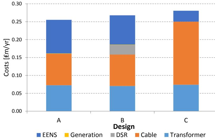
Figure 9.5: Cost components of risk-neutral (A) and two risk-averse design alternatives (B and C)
