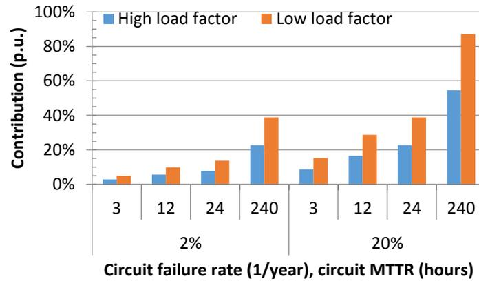
Figure 4.15. Impact of load profile on contribution
