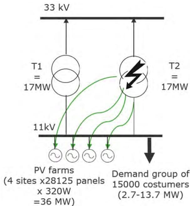
Figure 9.13: Test system including a protection system to reduce post-fault overloads
