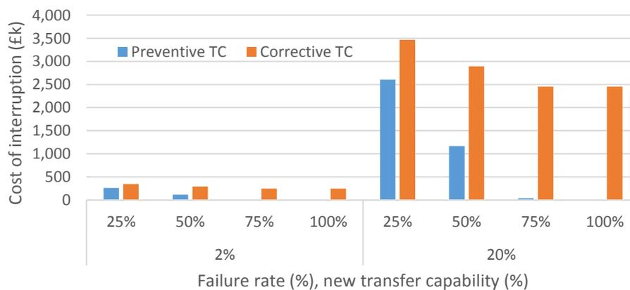
Figure 3.12. Total cost of preventive and corrective transfer capability
