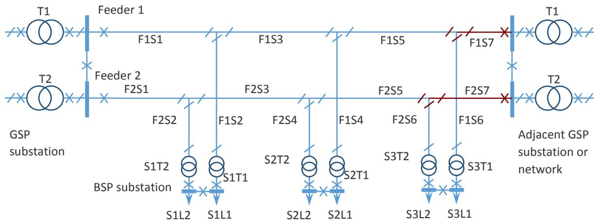
Figure 11.25: 132 kV generic network configurations
