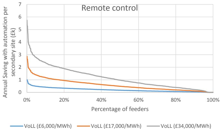
Figure 7.5. Potential savings of remote control
