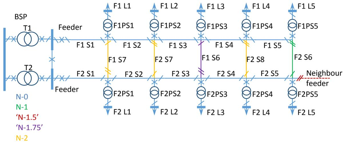
Figure 11.10: A generic EHV network system with different configurations to provide certain levels of security of supply
