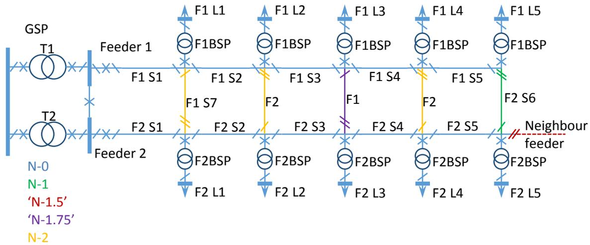
Figure 11.18: A generic 132 kV network system with different configurations to provide certain levels of security of supply
