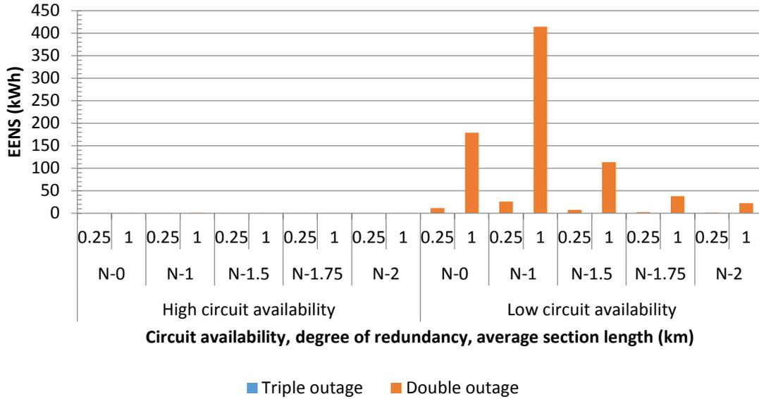
Figure 11.8: N-2 and N-3 components of EENS for different circuit availabilities, degrees of redundancy and section lengths for underground feeders with total feeder peak demand of 5,000 kW; linear Y-axis
