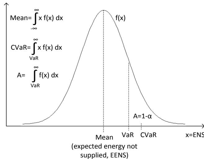
Figure 9.2: CVaR concept proposed for reliability analysis
