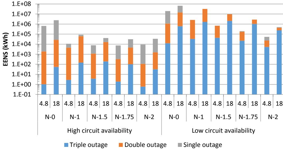
Figure 11.22: EENS for different circuit availabilities, degrees of redundancy and section lengths for underground feeders with total feeder peak demand of 300 MW; logarithmic Y-axis
