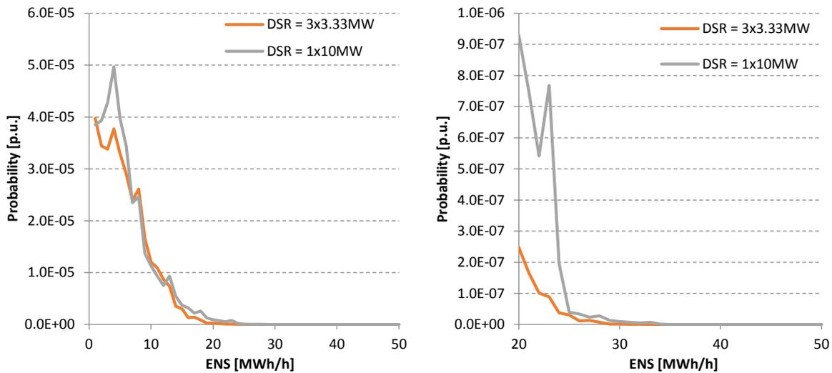
Figure 9.7: ENS PDFs of optimum risk-averse solution (3 DSR facilities, solution D) and alternative design with 1 DSR facility (same net DSR volume), shown in the following ranges: (left)  $1 \leq \text{ENS} \leq 50$  and (right)  $20 \leq \text{ENS} \leq 50$ .
