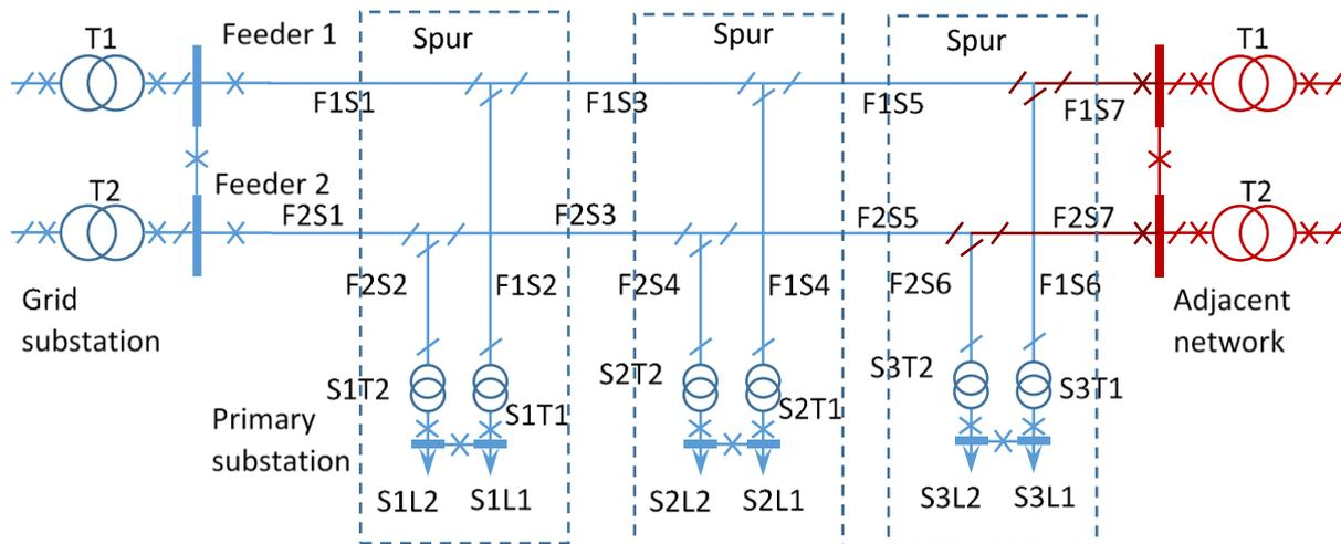
Figure 9.9: EHV Generic network configuration (illustrated for three primary substations) with optional connection to neighbouring grid substation
