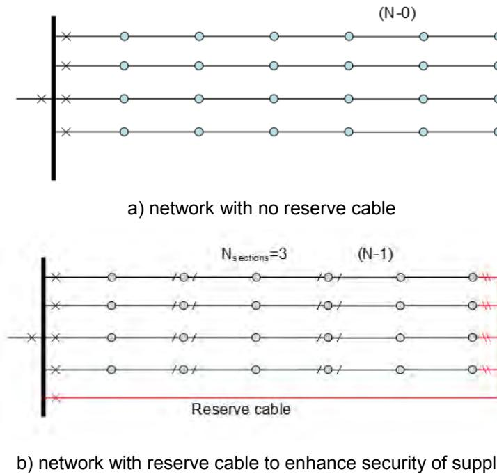
Figure 2.17: Test network a) without and b) with reserve cable
