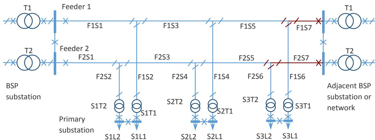
Figure 11.17: EHV Generic network configurations (Three Primary Substations Illustration)
