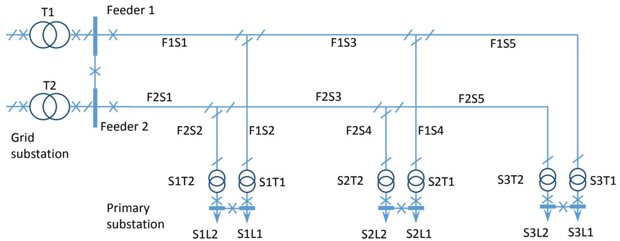
Figure 2.10: The topology of an EHV network with 3 primary substations used in the study
