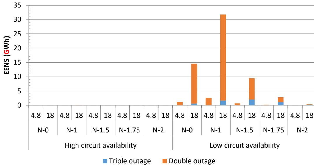
Figure 11.24: N-2 and N-3 components of EENS for different circuit availabilities, degrees of redundancy and section lengths for underground feeders with total feeder peak demand of 300 MW; linear Y-axis
