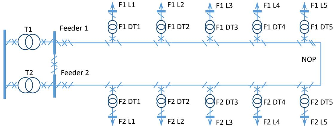
Figure 2.14: An example of radial HV distribution network
