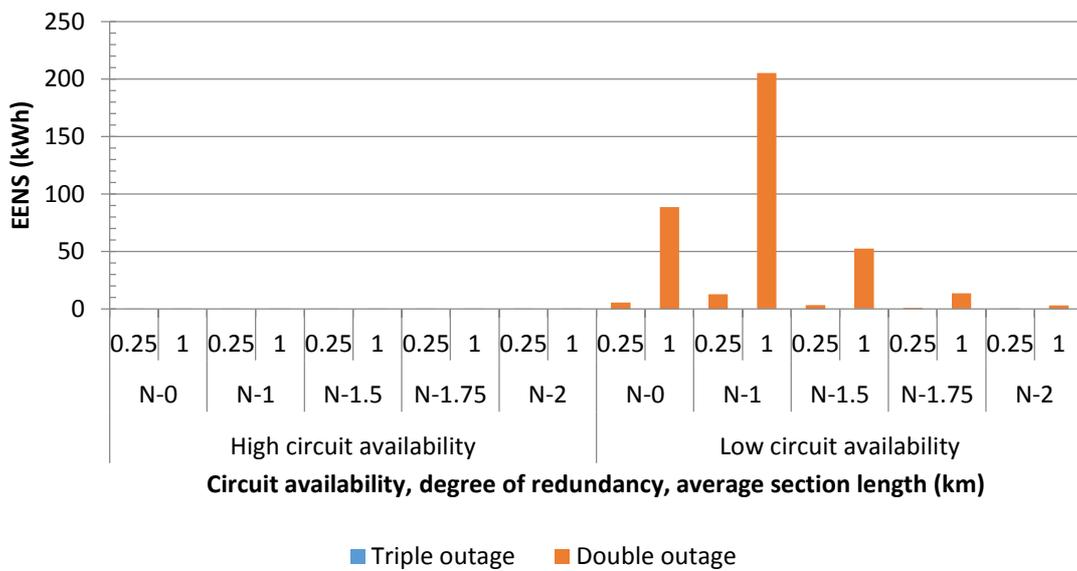
Figure 11.5: N-2 and N-3 components of EENS for different circuit availabilities, degrees of redundancy and section lengths for underground feeders with total feeder peak demand of 2,500 kW; linear Y-axis
