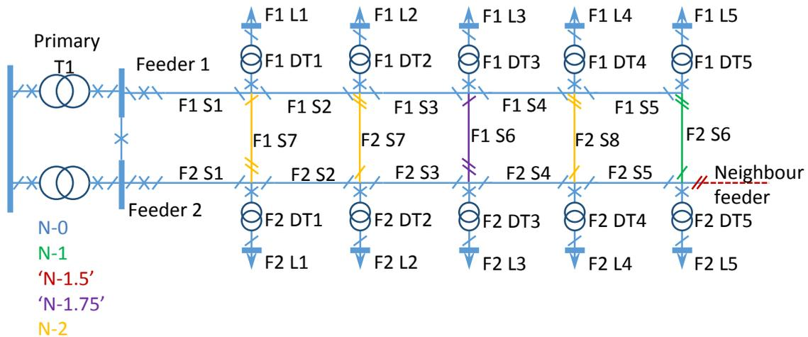
Figure 11.2: A generic HV network system with different configurations to provide certain levels of security of supply
