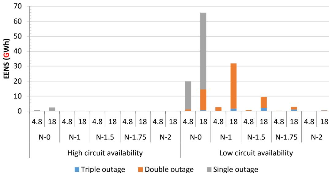
Figure 11.23: EENS for different circuit availabilities, degrees of redundancy and section lengths for underground feeders with total feeder peak demand of 300 MW; linear Y-axis
