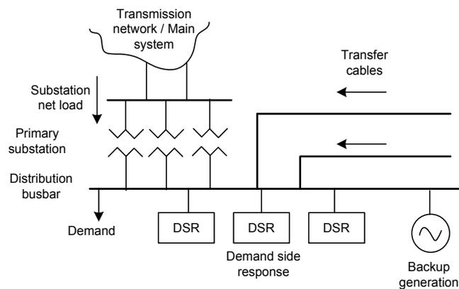
Figure 9.1: Diagram of primary substation with candidate technologies
