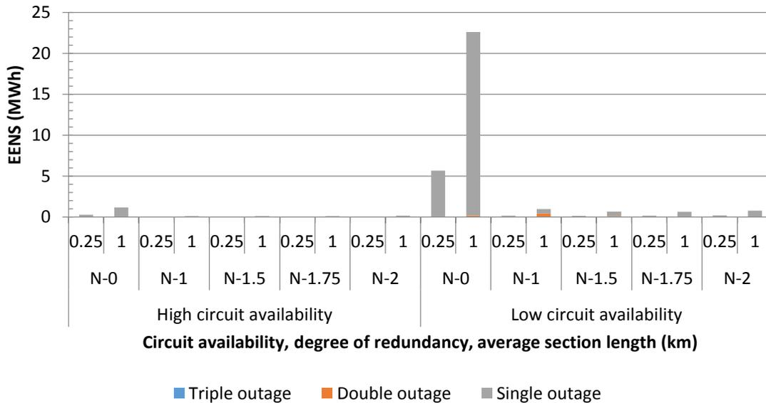
Figure 11.7: EENS for different circuit availabilities, degrees of redundancy and section lengths for underground feeders with total feeder peak demand of 5,000 kW; linear Y-axis
