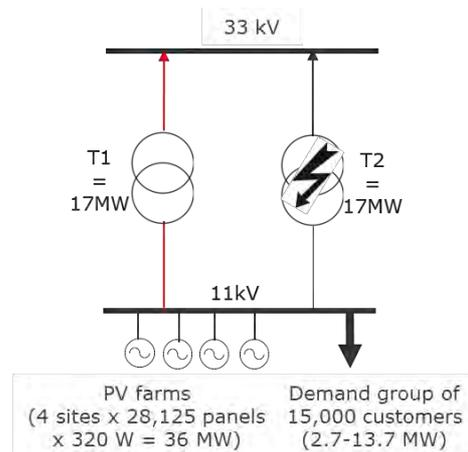
Figure 5.1: Test network. A failure in T2 (T1) in combination with reverse flows may overload T1 (T2)
