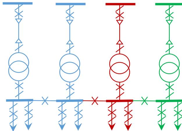
Figure 2.3: Illustration of primary two-transformer (blue), three-transformer (including red) and four-transformer (including green) primary substations
