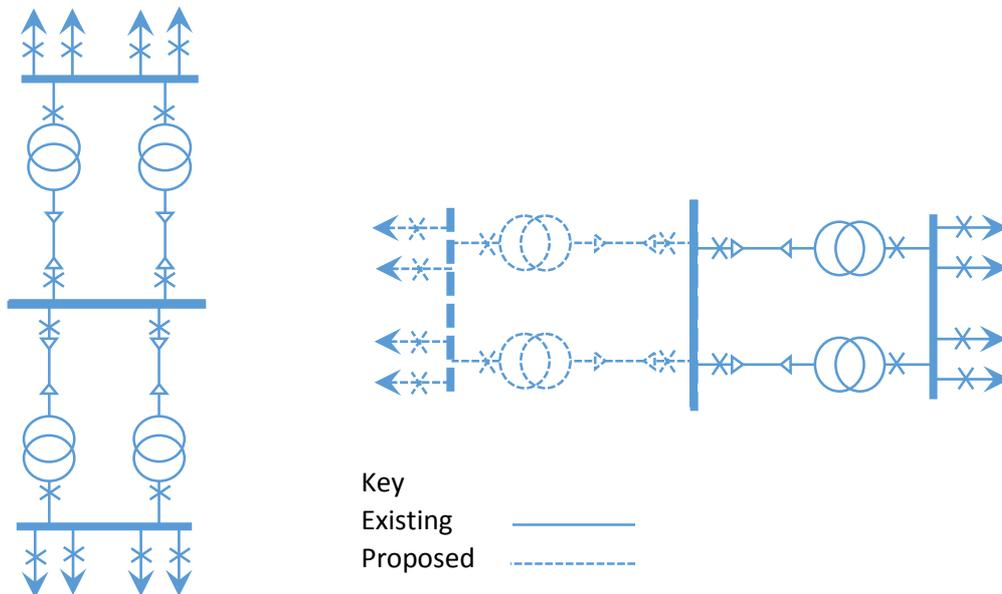
Figure 2.8. Schematic layout of 33/11 kV substations
