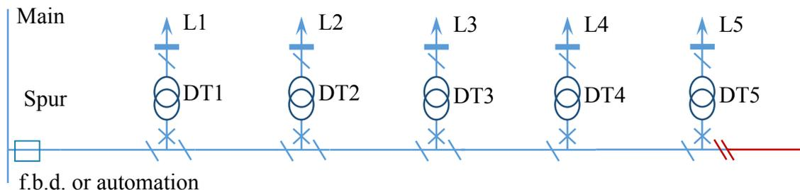
Figure 2.9: The topology of a HV spur used in the study with an option to improve security by adding a back-feed connection
