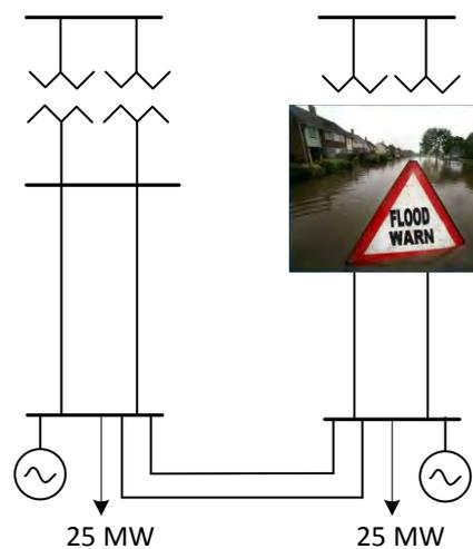
Figure 9.24: Location of demand and entry points together with configuration of candidate infrastructure (i.e. backup generation and candidate lines that can be built in preventive –upfront- or corrective mode)
