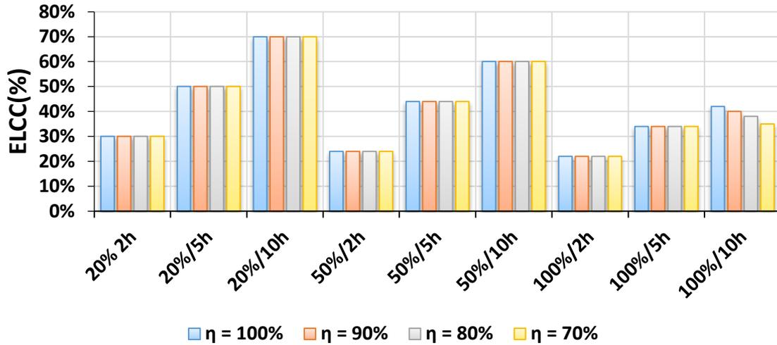
Figure 4.41: Normalized ELCC for nine storage plants across four efficiency levels. MTBF = 1 year, MTTR = 12 hours.
