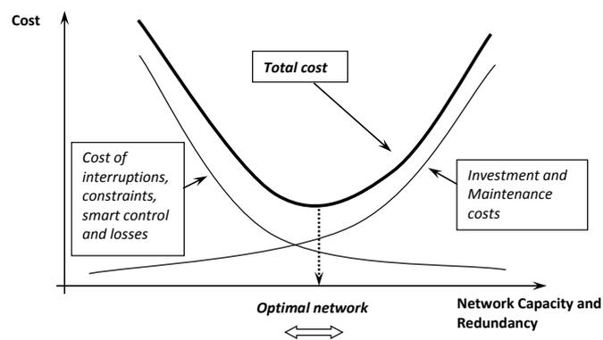
Figure 2.12: Balancing of network investment costs against customer interruption costs for network planning
