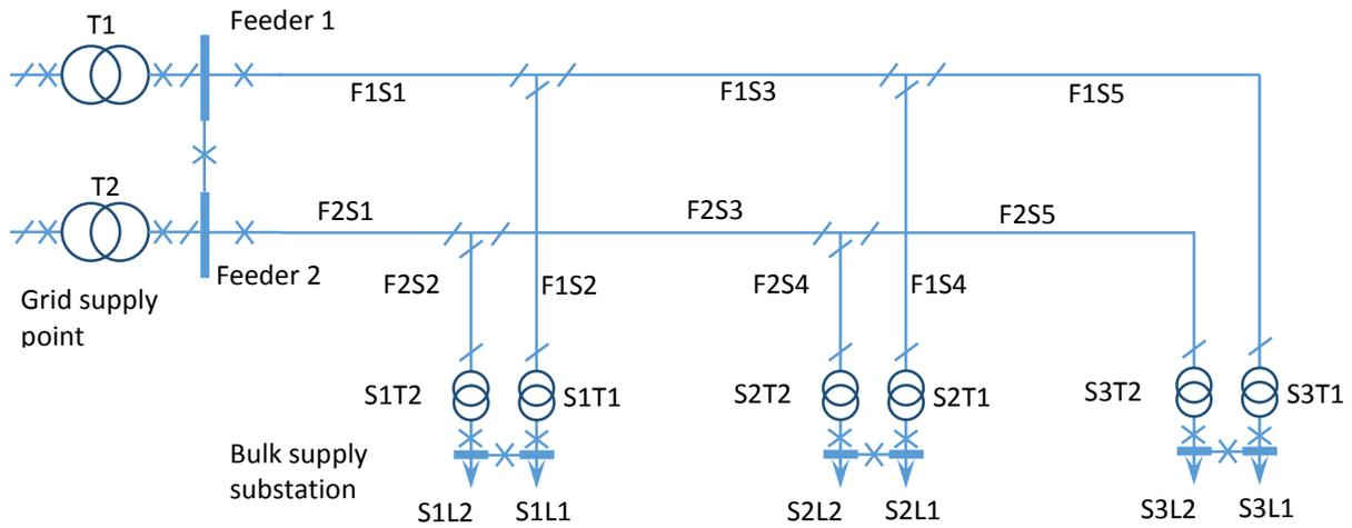
Figure 2.11: The illustrative topology of a 132 kV network with 3 bulk supply substations used in the study
