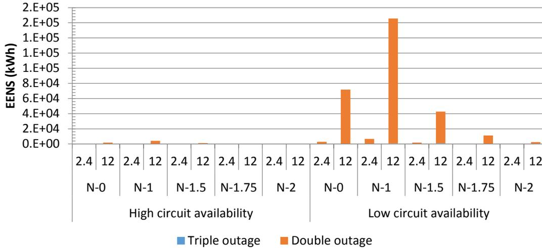
Figure 11.16: N-2 and N-3 components of EENS for different circuit availabilities, degrees of redundancy and section lengths for underground feeders with total feeder peak demand of 100 MW; linear Y-axis
