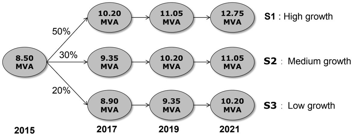
Figure 8.2: Scenario tree showing evolution of peak demand and transition probabilities for each scenario.
