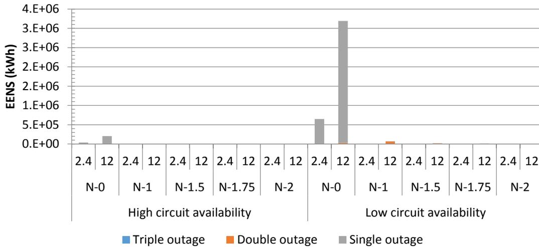
Figure 11.12: EENS for different circuit availabilities, degrees of redundancy and section lengths for underground feeders with total feeder peak demand of 37.5 MW; linear Y-axis
