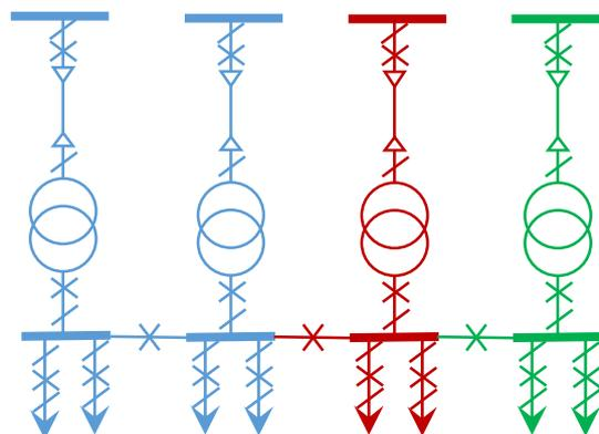
Figure 11.9: Illustration of primary two-transformer (blue), three-transformer (including red part) and four-transformer (including red and green part) primary substations
