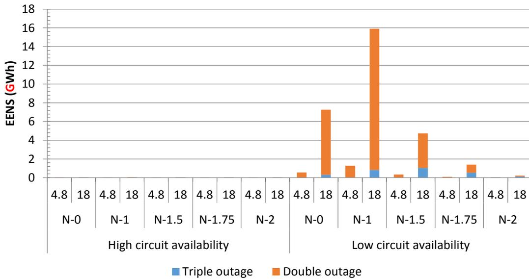
Figure 11.21: N-2 and N-3 components of EENS for different circuit availabilities, degrees of redundancy and section lengths for underground feeders with total feeder peak demand of 150 MW; linear Y-axis
