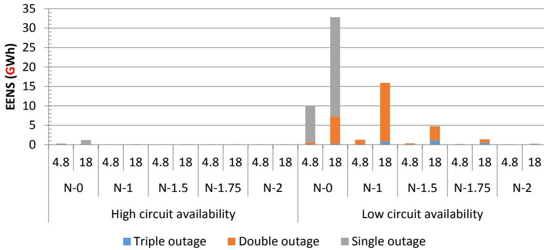
Figure 11.20: EENS for different circuit availabilities, degrees of redundancy and section lengths for underground feeders with total feeder peak demand of 150 MW; linear Y-axis
