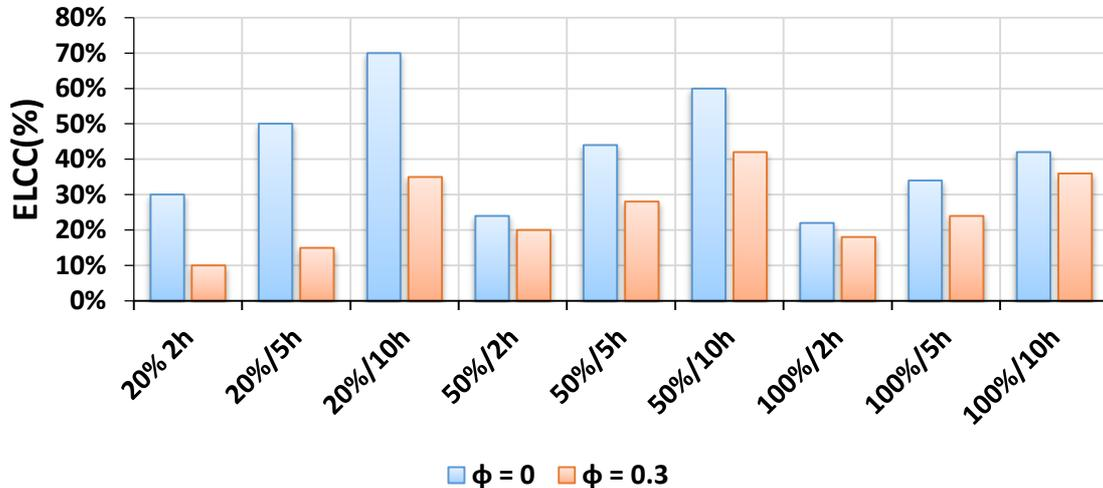
Figure 4.43: Normalized ELCC for nine storage plants across three demand shapes under N-1. MTBF = 1 year, MTTR = 12 hours.
