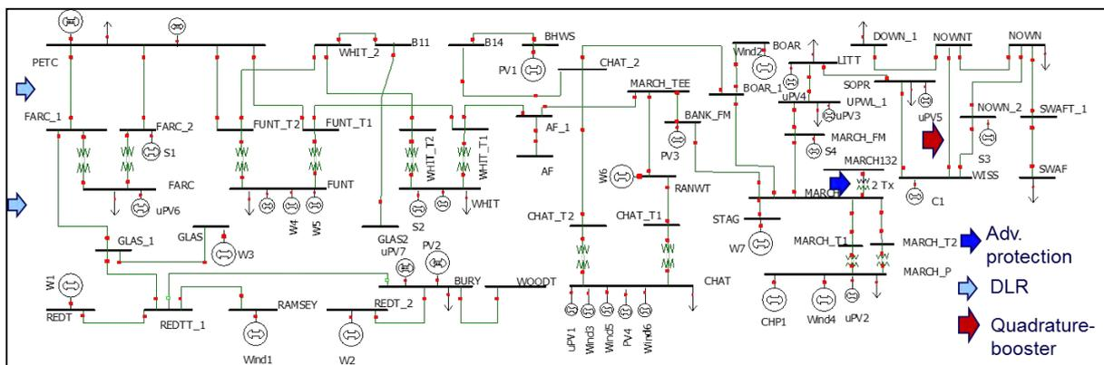
Figure 6.17. Smart solution to improve network utilisation
