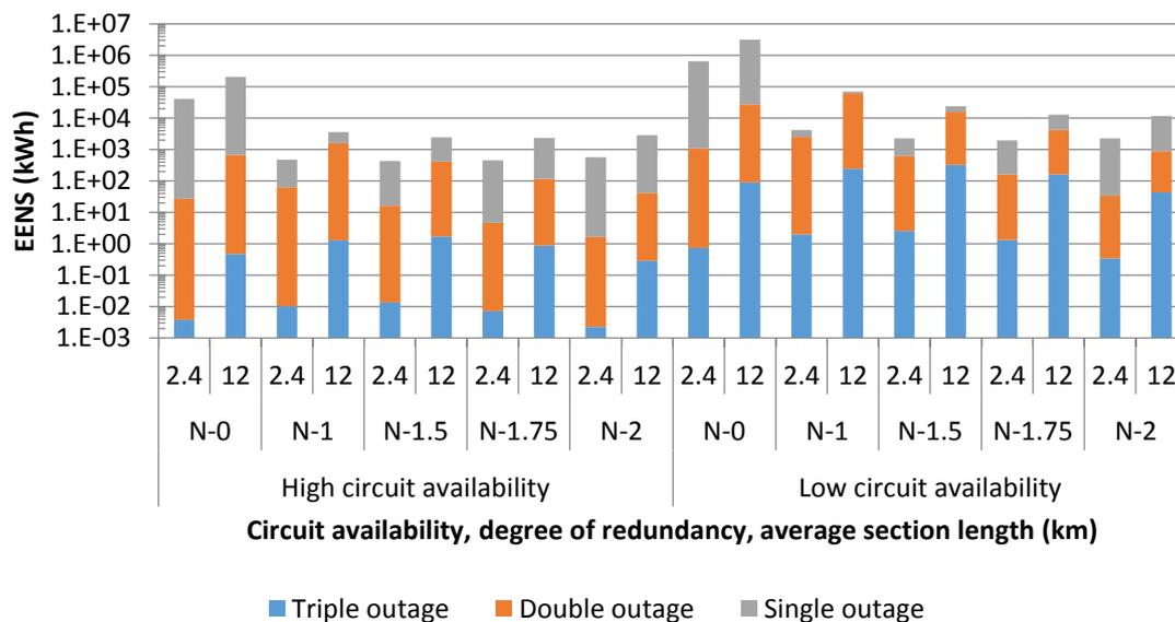
Figure 11.11: EENS for different circuit availabilities, degrees of redundancy and section lengths for underground feeders with total feeder peak demand of 37.5 MW; logarithmic Y-axis
