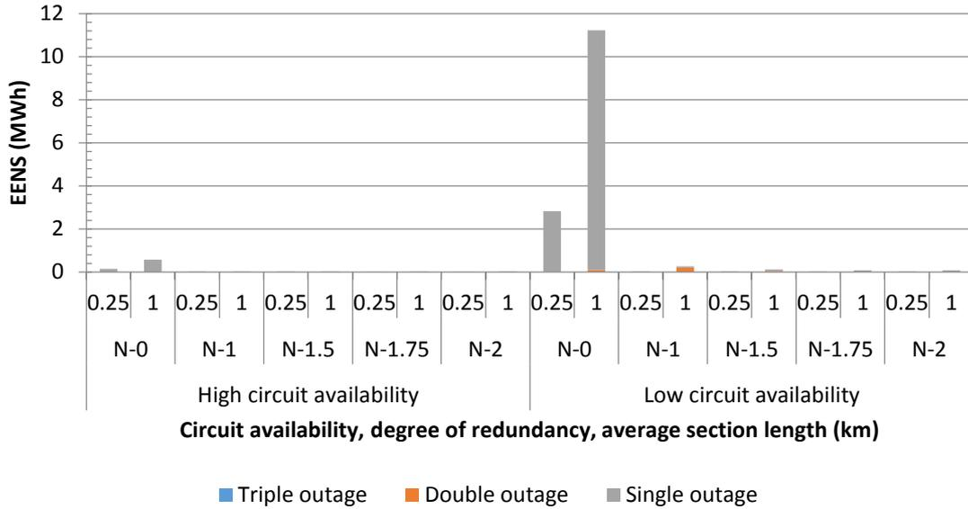
Figure 11.4: EENS per annum for different circuit availabilities, degrees of redundancy and section lengths for underground feeders with total feeder peak demand of 2,500 kW; linear Y-axis
