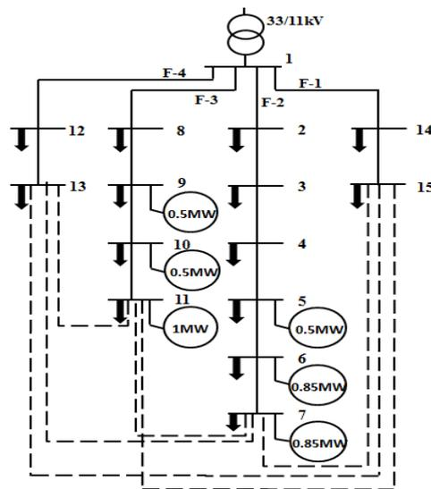
Figure 8.10: Diagram of the semi-urban 11 kV distribution network, showing prospective DG connections. Any section between two buses is considered to be a 1-km length distribution line.
