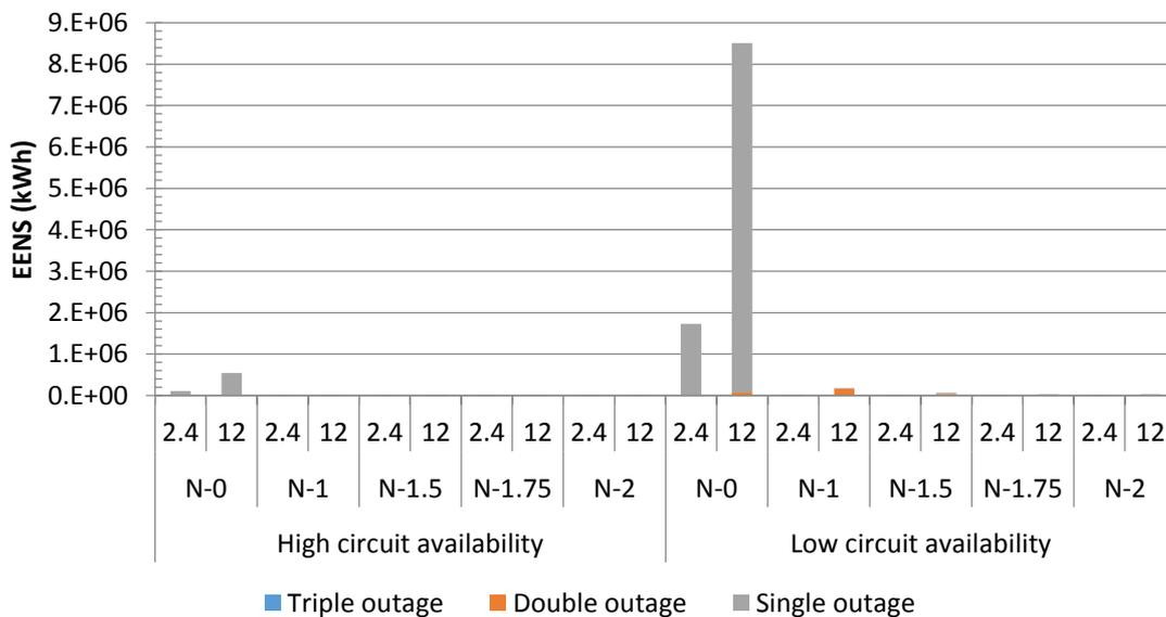
Figure 11.15: EENS for different circuit availabilities, degrees of redundancy and section lengths for underground feeders with total feeder peak demand of 100 MW; linear Y-axis
