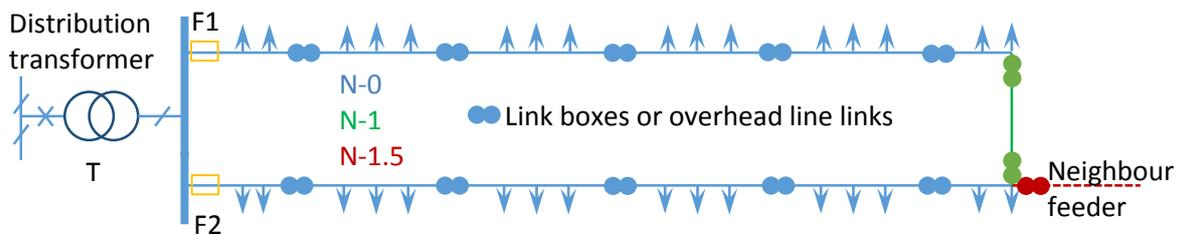
Figure 11.1: A generic LV network system with different configurations to provide certain levels of security of supply
