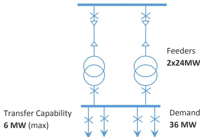
Figure 2.6. Dual-circuit transformer-feeder system
