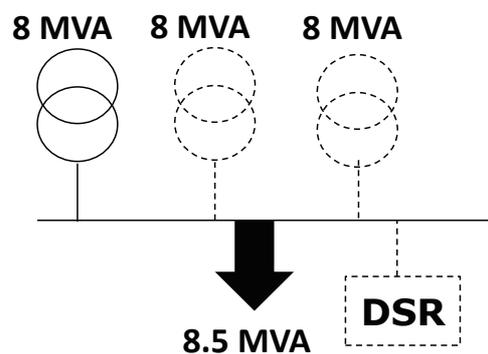
Figure 8.1: Distribution system under study (dotted lines show candidate investments to reinforce the network).
