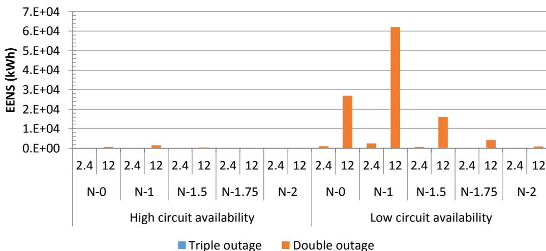
Figure 11.13: N-2 and N-3 components of EENS for different circuit availabilities, degrees of redundancy and section lengths for underground feeders with total feeder peak demand of 37.5 MW; linear Y-axis
