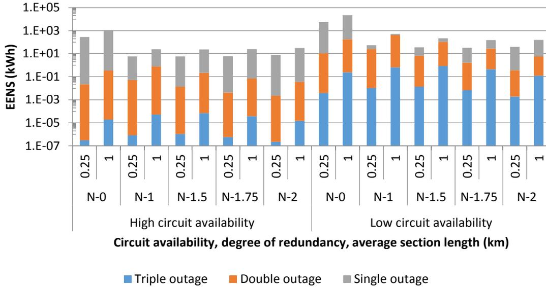
Figure 11.6: EENS for different circuit availabilities, degrees of redundancy and section lengths for underground feeders with total feeder peak demand of 5,000 kW; logarithmic Y-axis
