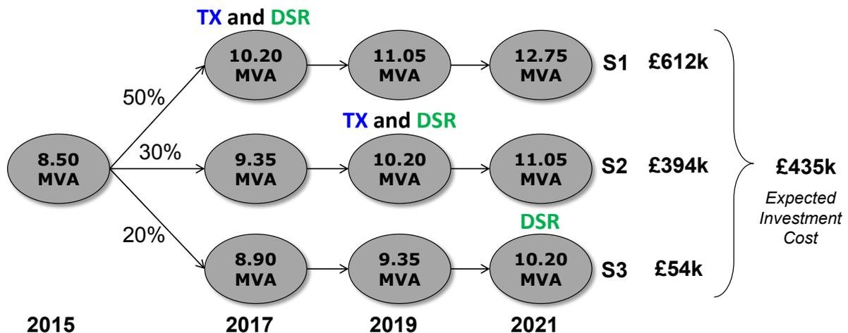
Figure 8.5: Optimal stochastic investment strategy when the planner can build both conventional and DSR assets.
