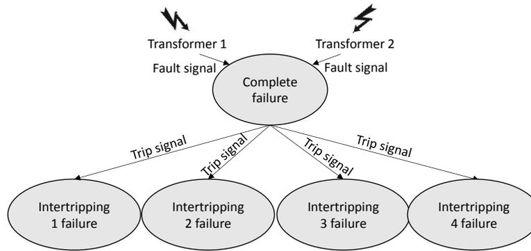
Figure 9.14: Failure model diagram of the protection scheme
