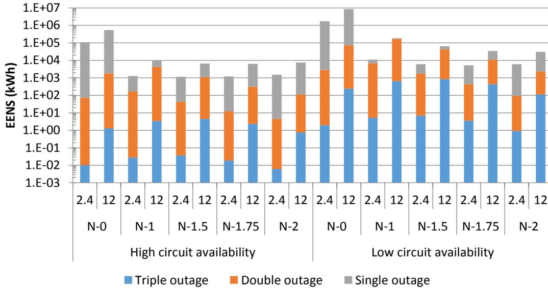
Figure 11.14: EENS for different circuit availabilities, degrees of redundancy and section lengths for underground feeders with total feeder peak demand of 100 MW; logarithmic Y-axis
