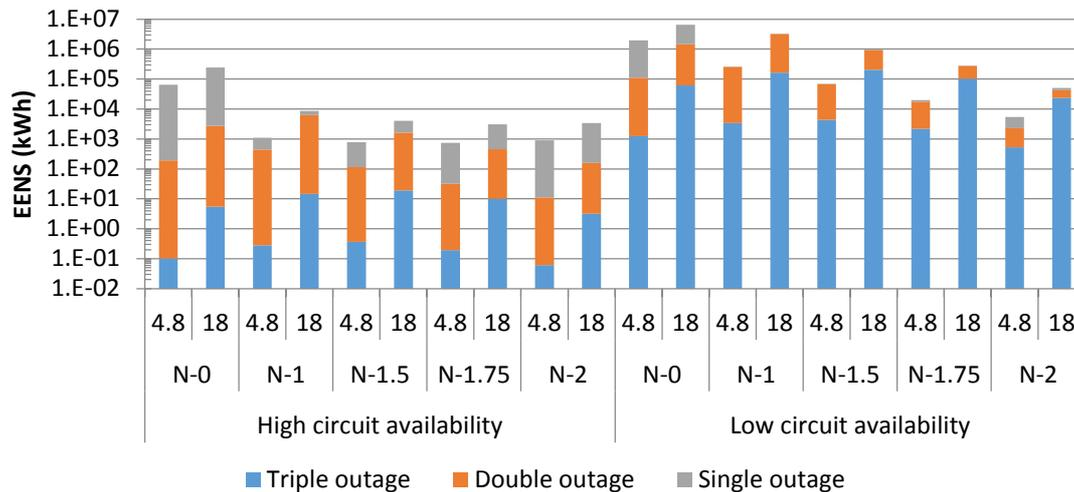
Figure 11.19: EENS for different circuit availabilities, degrees of redundancy and section lengths for underground feeders with total feeder peak demand of 150 MW; logarithmic Y-axis
